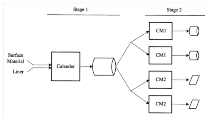
Figure: Two Stages Manufacturing System. (Lin and Liao 2003)
